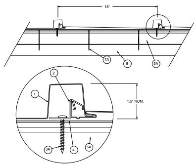
Metal Roof Deck Panels\* - No. 24 MSG min coated steel panels, 18 in. wide, \_ in. high at female side rib and 1-1/2 in.
